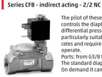
The pilot of these indirect acting solenoid valves controls the diaphragm position through a differential pressure. These valves are therefore particularly suitable for controlling high fluid flow rates and require very low working pressures to operate.
